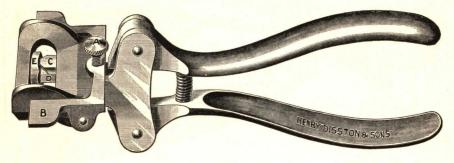
The idea embodied in this Saw-Set is one that will commend itself to every user of a saw-setting tool. The principal feature is the use of two plungers operated by the two levers or handles; pressure on the lower lever forcing plunger "D" against the body of the saw, thus holding it rigidly in position and preventing slipping, whilst a continuation of the pressure on the upper lever operates plunger "C" in setting the tooth.
